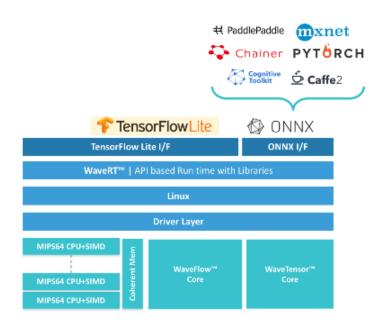
The TritonAl 64 APK provides for a TensorFLow-Lite framework stack running on a Linux OS
